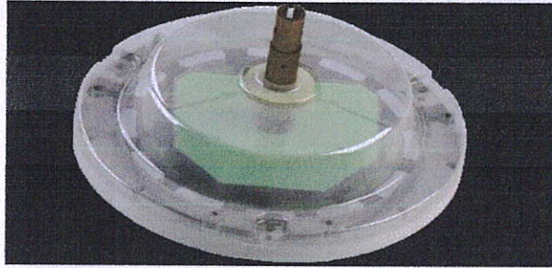
Figure 15: BLDC motor of Energy Efficient fan
